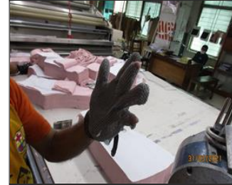
Photo of non-conformity Findings 7.6 - Metal hand glove found torn.JPG
