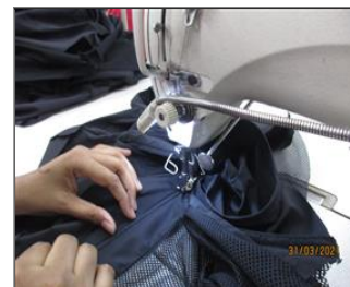
Photo of non-conformity Findings 7.17 - Needle guard displaced.JPG
